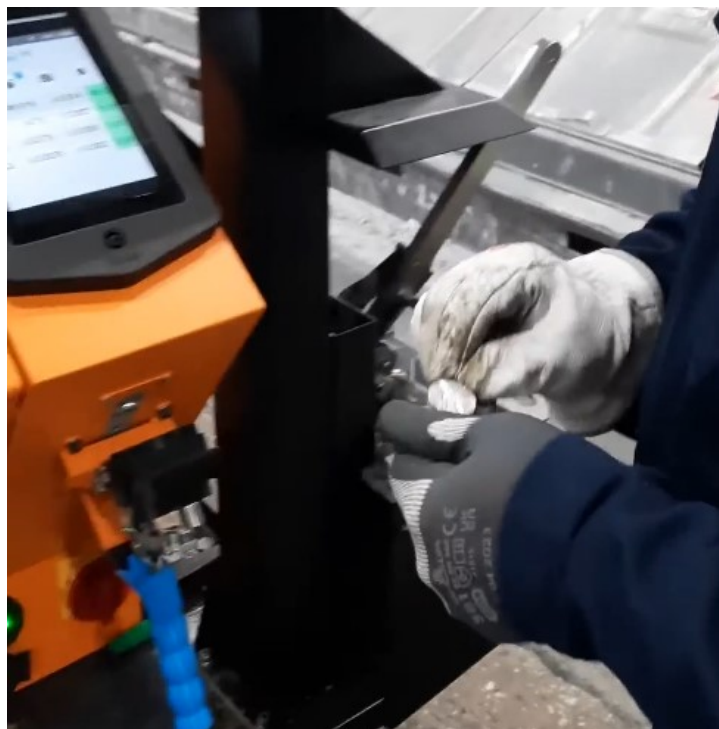
Figure 5. Showing the clean and homogeneous sample being loaded into the analyser.
