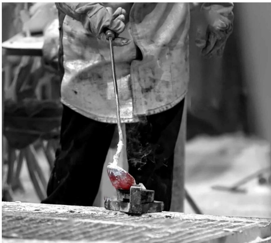
Figure 1. Showing an operator pouring liquid aluminium into a mould at the smelter.
