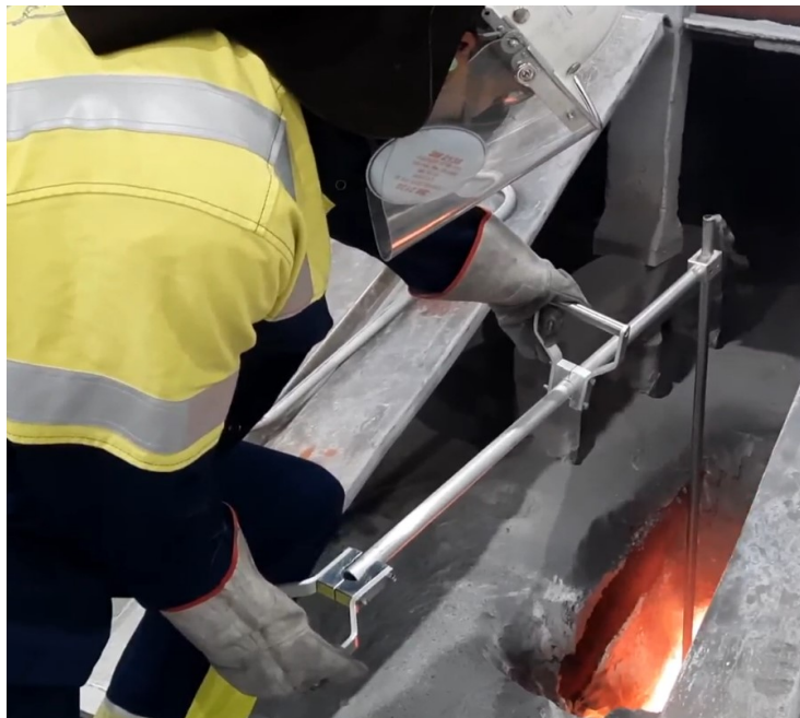
Figure 3. Showing the sampler being immersed in the smelter pot.
